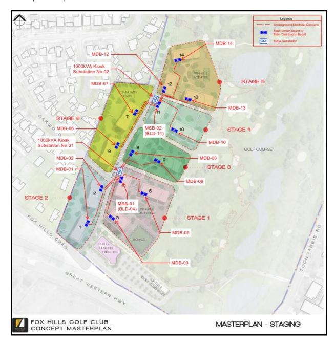
Preliminary analysis indicates that at present the existing network could have available capacities to cater for the required load demand 2MVA with N-1 supply security.
